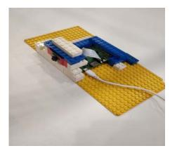
Fig. 3. The PI Camera and RPi set up in a Lego Structure to keep a steady
