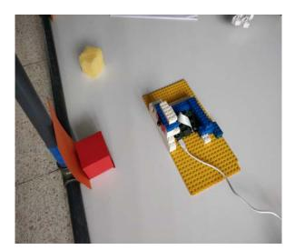
Fig. 4. The PI Camera and RPi set up at a distance from the red cube
