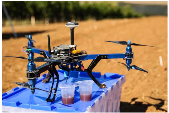
Fig. 5. Multicopter from 3D Robotics, mainly used for ripeness analysis
