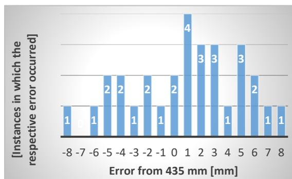
that the distance the engine travels fluctuates. The diagram below is a result of the documentation that had to be written in the course of the Botball competition. It shows the fluctuations the travel of the engines has at a certain distance.
