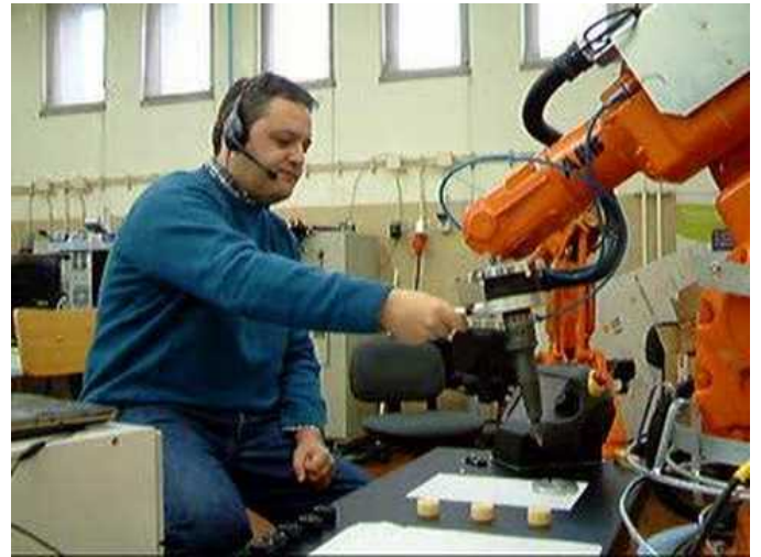
Fig. 5. An industrial robot is trained by an operator ( https://www.youtube.com/watch?v=IXSho9loGYU )
