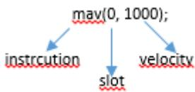
So that you can program the robot to drive a curve you have to let one motor drive faster than the other one.
