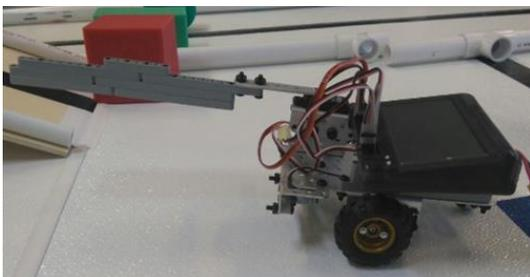
The second robot was not as simple to construct as the first one. With both of the robots we tried many other types of effectors, but we were not able to convert most of our ideas into reality because their implementation was too complex and complicated for us as "beginner mechanical engineers". So we decided to build only simple effectors. On the second robot we used gears to construct an effector. This effector takes the red Botnout, draws the Lego-blocks together which were
