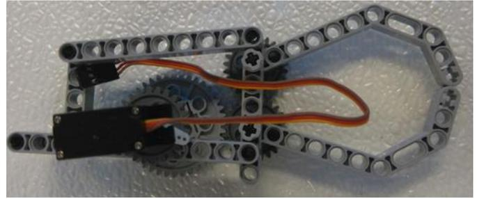
At first our second robot had a different crew arm. This crew arm was made out of metal bits and one servo. But this construction was too long and we couldn't get up to the crater rim. Together with the other robot it didn't fit into the starter box, so we had to abandon this idea.
